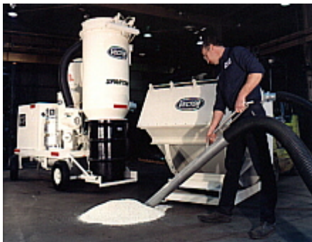
Spartan II Vacuum Working With Optional Self-Dumping Two Yard Hopper
