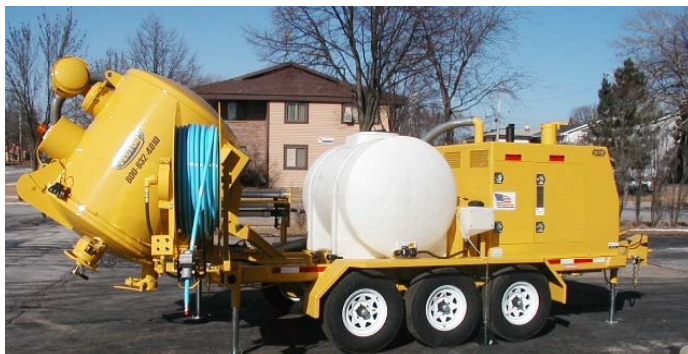
Super Neptune to 3,400 CFM and 35 GPM Jetter
