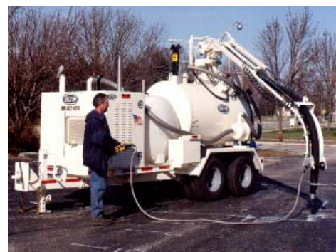
Super Neptune to 3,400 CFM and 35 GPM Jetter
