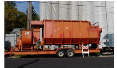
Titan MDCTM Mobile Dust Collectors Diesel, Electric/ Portable, Stationary 2,500 – 60,000 CFM
