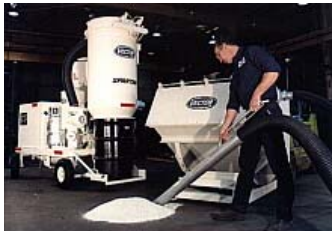
VecLoader Spartan® II Series Compact and powerful vacuums. Load into hoppers, drums, or other devices.
