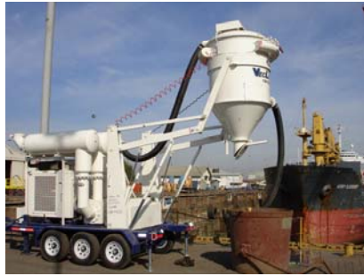
VecLoader Titan® 721 Series Versatile trailer units with the power of a vacuum truck.
