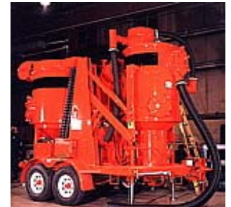
Titan Klean Shot™ Series Shot or Grit Reclaim System Combine with any Vacuum
