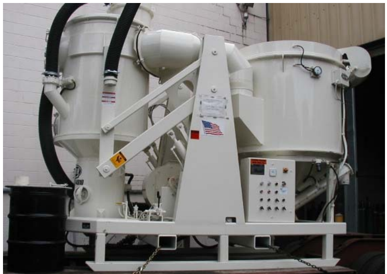
Skid Mounted Electric Klean Shot in Travel/Stowed Position
