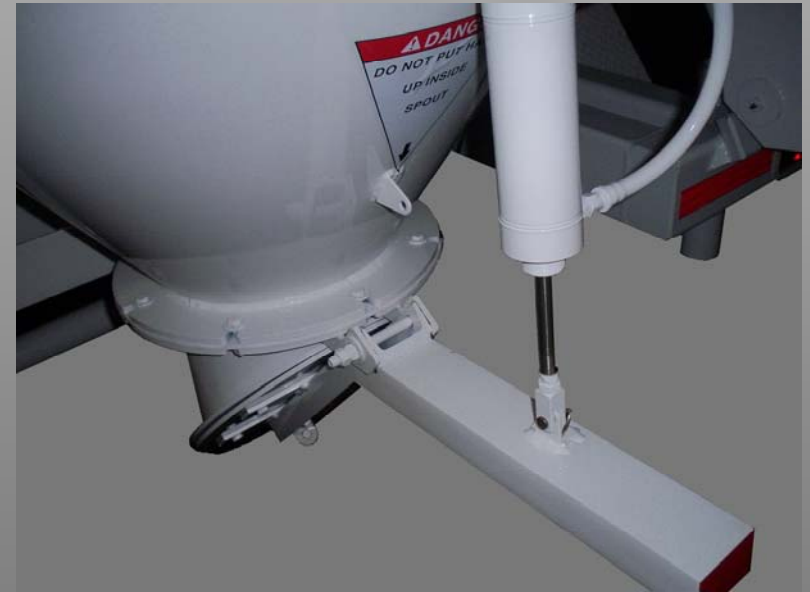
Standard Gravity Dump Door with Pneumatic Assist
