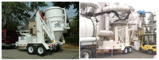
Standard Components on Trailer Gravity Dump Cyclonic Separator - 54" Diameter Design, Other Diameters Available
