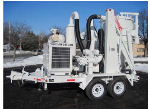
Side View of Catalyst Nitrogen Vacuum
