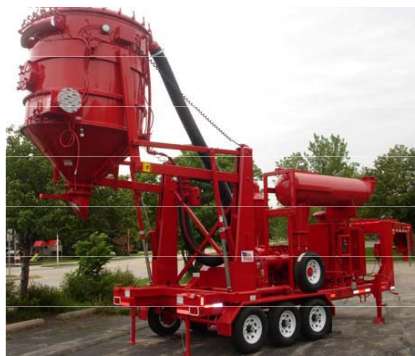
Hopper in Partially Raised Position Optional Gooseneck Trailer
