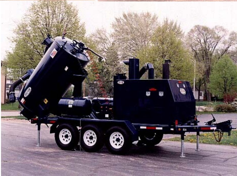
HydroVac 170D/1000 Shown (170 Horsepower Diesel, 1000 Gallon Storage)
