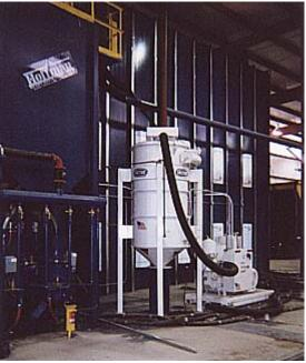
BH Series Cyclonic Baghouses/Collector Devices are configured in modular format for matching to Vector Technologies PM Series Power Modules or alternative vacuum sources to meet specific filtration and unload requirements. Units are set on legs at customer designated heights feature tangential inlets, deflector plates, removable wear plates, pulsed-cleaned Teflon coated filters, plus magnehelic gauges for filter monitoring.
